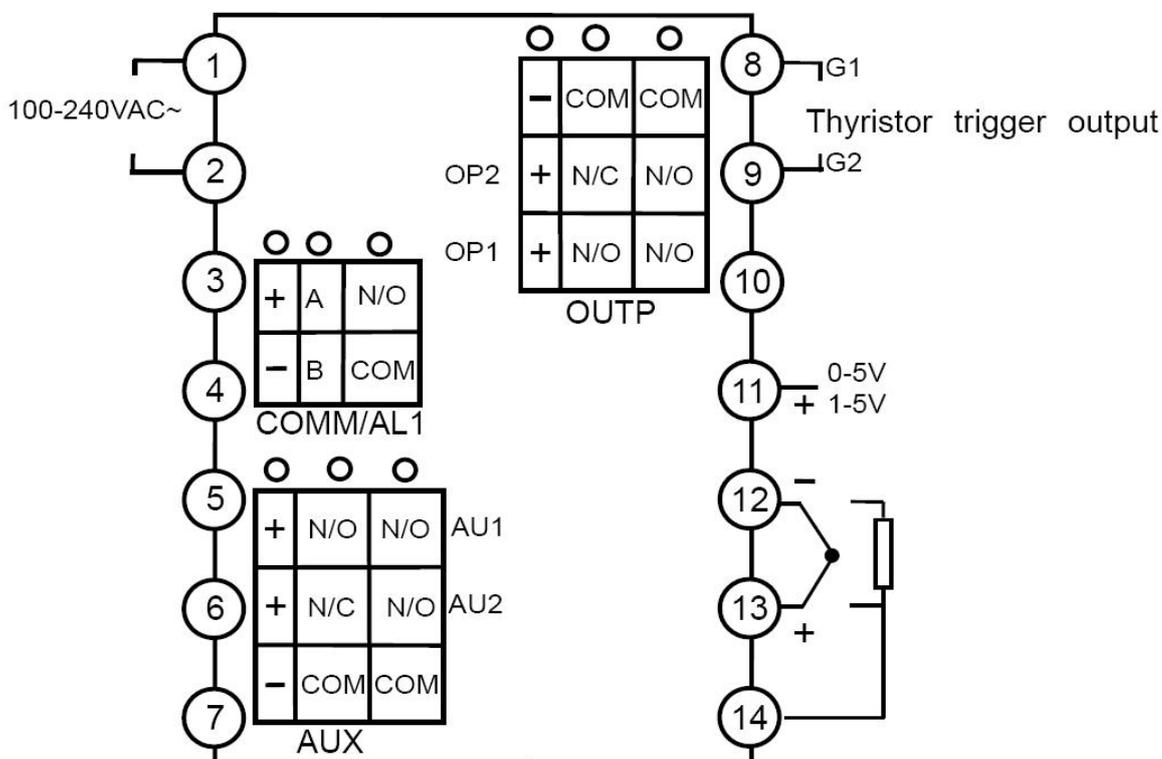
**Wiring graph of instruments with D2 dimension as below:**
