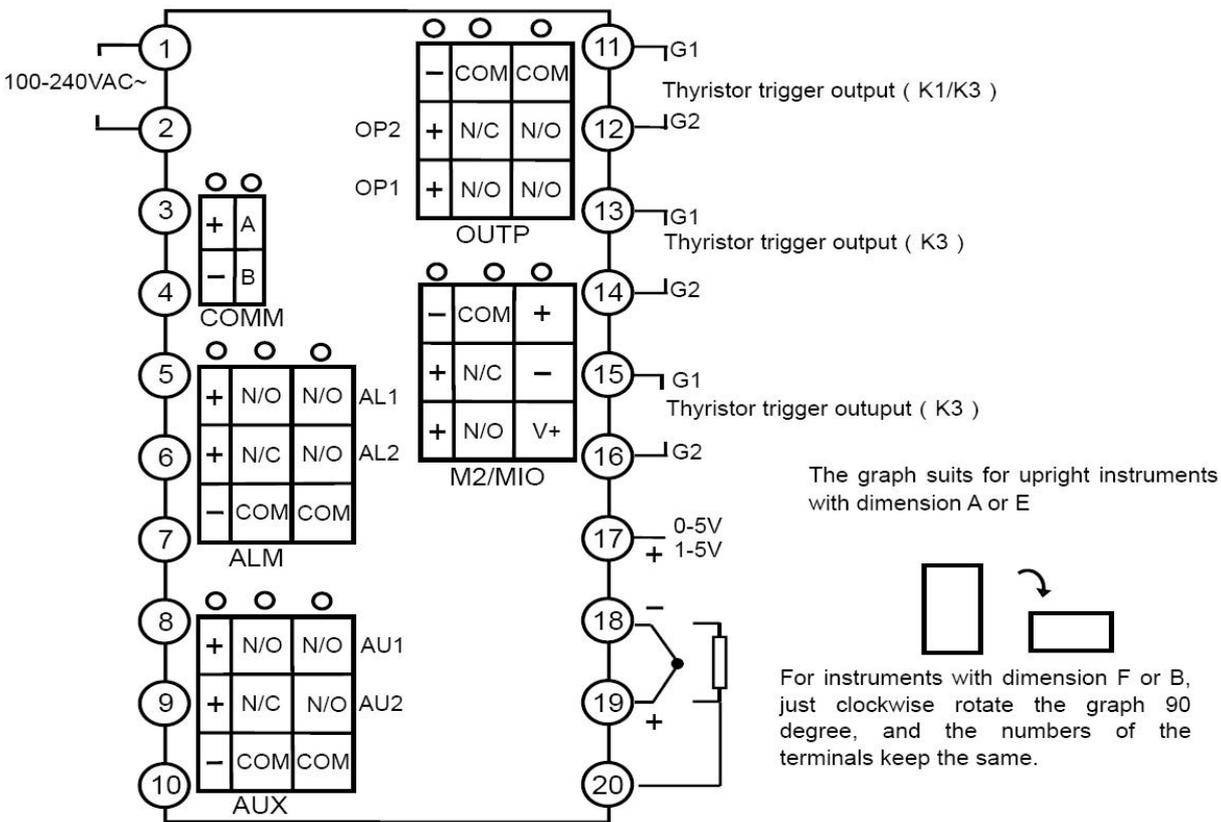
**Wiring graph of D dimension instruments (72x72mm)**
