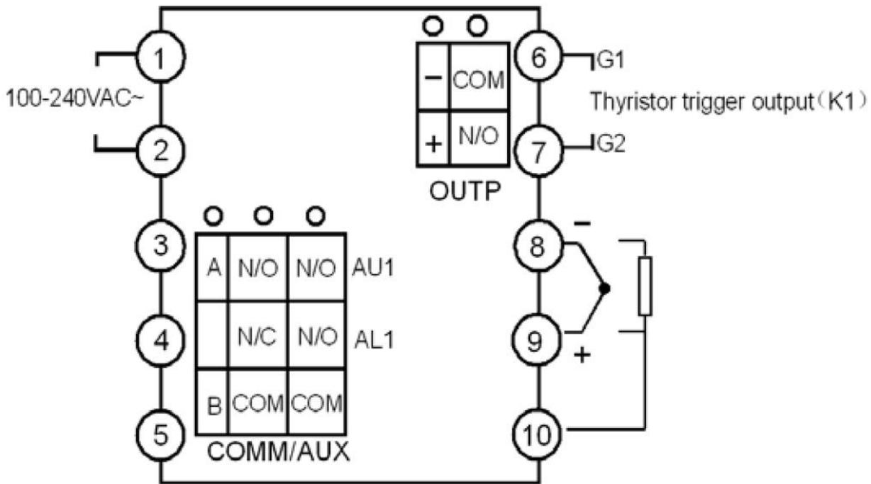
**Wiring graph of instruments with D5 dimension as below:**
