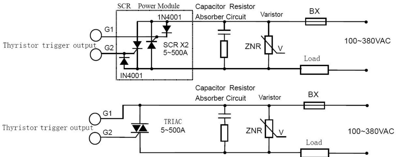
Note 1: According to the voltage and current of load, choose a suitable varistor to protect the thyristor.
